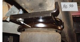
Left hand assembly (driver's side) attached with carriage bolts (R), flat washers (M) and nylon lock nuts (U). Torque to 31 lb.-ft. (42Nm).
