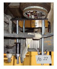
Right side (passenger's) view towards front of finished installation torqued to 10 lb.-ft. (14Nm).
