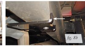
RH (passenger's) side. Push bracket against frame and torque to 38 lb.-ft. (52Nm).
