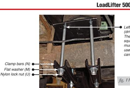
Left side (driver's side): The inside square holes must be used for the carriage bolts.
