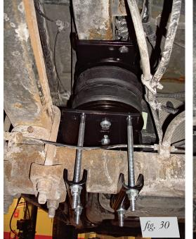
Left side (driver's): rear view of installation.
