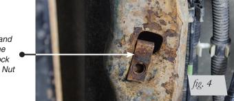
4. For the early 04-08 models, install a new Universal Nut (V) into the large hole so that
