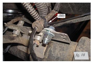
Left side (driver's): set one of the lower brackets on the axle making sure the inside leg is outboard (leaf spring side) of the ABS line bracket on the axle (Figs. 19 & 20). It may be necessary to angle the lower bracket into position. Make sure the lower bracket is pushed against the leaf spring and in between the stock U-bolts.
