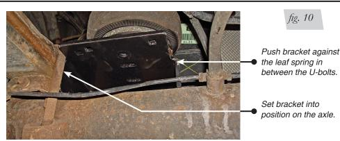
2. Left side (driver's) installation: insert the long carriage bolts (T) into the bottom bracket.
