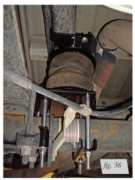
Right side (passenger's): front view of installation.
