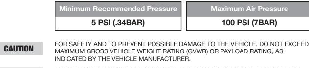
**CAUTION** ALTHOUGH THE AIR SPRINGS ARE RATED AT A MAXIMUM INFLATION PRESSURE OF 100 PSI (7BAR), THE AIR PRESSURE ACTUALLY NEEDED IS DEPENDENT ON LOAD AND GROSS VEHICLE WEIGHT RATING.
