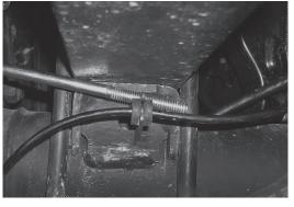
*fig. D.13* U-bolt in position for use on the lower bracket.
