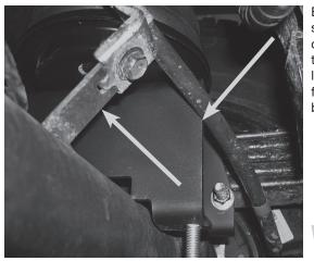
Bend the bracket slightly to gain clearance between the emergency brake line and lower bracket forward of the axle on both sides.
