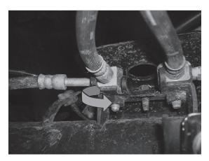
Loosen the bolt holding the brake line to the axle bracket and rotate the brake line counterclockwise as far as it can go. Tighten the brake line bolt so the line stays in this position.
