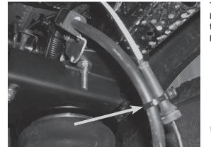
16. Tie off the ABS line on the passenger's (right) side, which was disconnected from the axle bracket, to the axle vent tube with a tie strap (U) (Fig. D.31).
