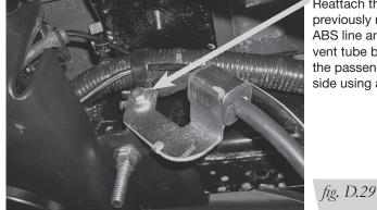
Reattach the previously removed ABS line and axle vent tube bracket on the passenger's (right) side using a P-clamp.
