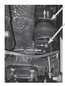
Push the air spring forward or backward and tighten the mounting hardware.
