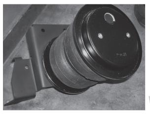
4. Install the lower brackets (A) onto the air spring assemblies with two 3/8"-16 x 7/8" hex-cap screws (F), 3/8" lock washers (G) and 3/8" flat washers (H) (Fig. D.18), making sure that the flanges on the lower brackets face the fittings on the top of the air springs. (Fig. D.19).
