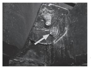
5. Remove the ABS lines from the brackets on the driver's (left) and passenger's (right) side axle (Fig. D.5).
