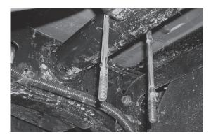
Set the round U-bolts around the cross member over the axle, as shown, on both driver's (left) and passenger's (right) sides. Be careful not to pinch any wiring that may be in the area on the driver's (left) side.
