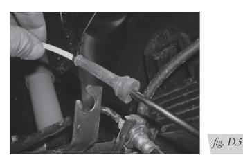
6. On the driver's (left) side line, loosen the left bolt that holds the rear brake line to the rear axle bracket. Rotate the brake line counter clockwise as far as it will go. Tighten the brake line bolt so the line stays in this position (Fig. D.6). This is done to gain clearance for the lower bracket.
