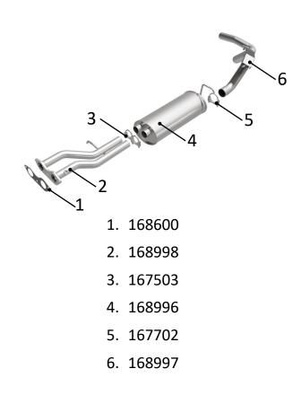
(Carefully read all instructions before installation) Disconnect the vehicle's battery before removal of the OEM exhaust system. This will prevent electrical accidents and will reset the computer if it applies to the vehicle. Remove existing exhaust system from the vehicle. Only remove parts that will be replaced. Clean existing flange with a wire brush to ensure proper sealing.
