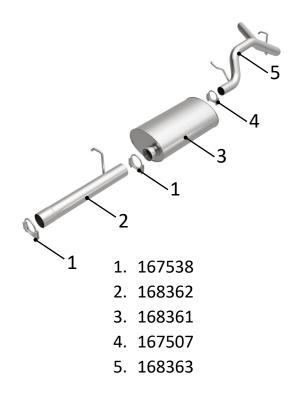
(Carefully read all instructions before installation) Disconnect the vehicle's battery before removal of the OEM exhaust system. This will prevent electrical accidents and will reset the computer if it applies to the vehicle. Remove existing exhaust system from the vehicle. Only remove parts that will be replaced. Clean existing flange with a wire brush to ensure proper sealing.
