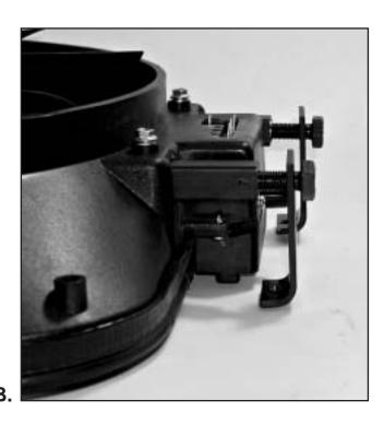
The included bracket (see image A) is used for the overflow tank. Using your original screws, mount the bracket to your radiator. Using the angle brackets (see image B) attach your fan to the top of the radiator, positioning it between the overflow tank and radiator tank.
