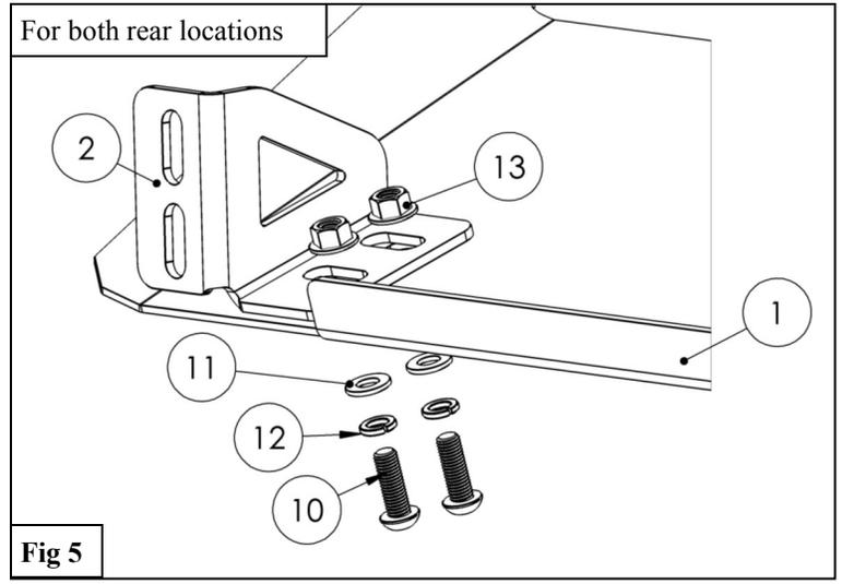
5. Align and tighten all hardware as specified: M8 to 18 ft-lbs, M10 to 38 ft-lbs.
