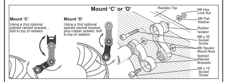
Two fans can be mounted side by side to provide a larger cooling area.
