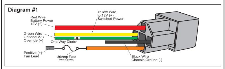
**RED Wire -** Attach to the Positive (+) Terminal of Battery
