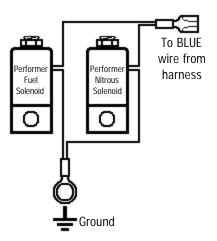
To test the wiring of your Performer Nitrous and Performer Fuel Solenoids, make sure that the bottle valve is in the "OFF" position. Turn the ignition key to the "ACC." position. With the arming switch in the "ON" position, quickly tap the microswitch button to activate the system. You should hear both solenoids "click" is wired correctly. Make sure that you perform this test with the valve OFF to prevent filling the manifold with Nitrous Oxide.
