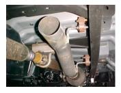
**2.** Install headpipe #A onto your catalytic converter and attach with clamp #H. Use a jack stand to support the converter. DO NOT TIGHTEN. Insert welded hangers into rubber grommets.
