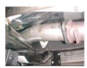
**6.** Re-install your catalytic converter to the new downpipe using your stock nuts and bolts. DO NOT TIGHTEN.
