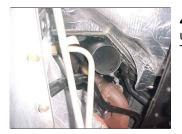
**4.** Install downpipe #J onto turbo using your stock clamp. DO NOT TIGHTEN.
