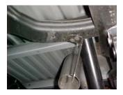
**6.** Remove the spare tire. On the passenger side rotate the bracket that holds the spare tire 180 degrees and re-install spare tire.
