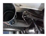
**7.** Install the exit pipe #D onto the over axle tailpipe and secure with clamp #G. DO NOT TIGHTEN. Insert welded hanger into rubber grommet
