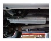
**4.** Install muffler #B onto headpipe 1½-2" with the louvers facing the converter. Secure with clamp #G. DO NOT TIGHTEN. Use a jack stand to support the muffler.
