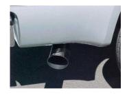
**8.** Install stainless steel tip #E. Clamp down. When you have everything in place, firmly tighten all bolts and clamps down securely. Use stainless steel cleaner and a Scotch Brite pad weekly to prevent tip from discoloration.
