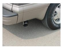
INSTALL YOUR STAINLESS STEEL TIP. USE ANY ALUMINUM OR STAINLESS STEEL CLEANER TO POLISH YOUR TIP. NOW FIRMLY TIGHTEN ALL CLAMPS, HANGERS AND FLANGES.
