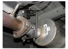
ATTACH FRONT MUFFLER HANGER #B TO MUFFLER INLET AND SLIDE HANGER INTO THE RUBBER GROMMET. THE VERTICAL PART OF THE HANGER WILL BE ON THE DRIVERS SIDE, DO NOT TIGHTEN.
