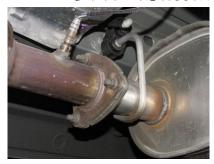
TO REMOVE STOCK EXHAUST UNBOLT IT FROM THE 3-BOLT FLANGE LOCATED JUST BEHIND THE CATALYTIC CONVERTER. YOU WILL REUSE YOUR FACTORY BOLTS.NOW CUT OFF YOUR STOCK TAILPIPE JUST BEHIND THE MUFFLER AND REMOVE. LEAVE FACTORY RUBBER GROMMETS IN PLACE. USE WD-40 TO AID IN REMOVAL OF EXHAUST AND HANGERS.
