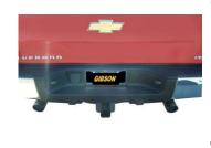
Install stainless steel tips. Clamp down. When you have everything in place, firmly tighten all bolts and clamps down securely. Use stainless steel cleaner and a Scotch Brite pad weekly to prevent tip from discoloration. Inspect all fasteners after 25-50 miles of operation and re-tighten as necessary.
