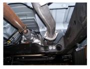
3. **2009/2010 Models Only** You will use part "N" to attach to the muffler re-using the factory clamp. Be sure that the tabs of the clamp are straight. If they are bent, it will not seal the connection.
