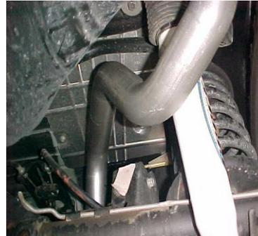
INSTALL THE OVERAXLE TAILPIPE #B INTO THE MUFFLER 1 1/2" TO 2". SECURE TO THE MUFFLER USING CLAMP #D. DO NOT TIGHTEN. INSERT WELDED HANGERS INTO RUBBER GROMMETS. NOTE, SHORT END OF OVER AXLE PIPE INSERTS INTO MUFFLER.
