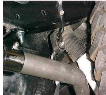
INSTALL STAINLESS STEEL TIP. CLAMP DOWN. WHEN YOU HAVE EVERYTHING IN PLACE, FIRMLY TIGHTEN ALL BOLTS AND CLAMP DOWN SECURELY. TO CLEAN STAINLESS TIP, USE A SCOTCH BRITE PAD AND ANY STAINLESS STEEL OR ALUMINUM CLEANER.
