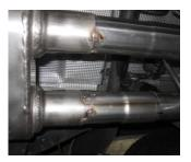
4. Install muffler #B onto headpipe #A 1.5-2". Use a jack stand to support the muffler. Use clamp #f to secure muffler to headpipe. Do not tighten.
