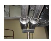
7. Install stainless steel tips. Clamp down. When you have everything in place, firmly tighten all bolts and clamps down securely. Inspect all fasteners after 25-50 miles of operation and re-tighten as necessary.
