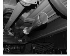
INSTALL HEADPIPE #A ONTO STOCK FLANGE, USE STOCK 15MM NUTS TO SECURE IT. DO NOT TIGHTEN, JUST MAKE SNUG.
