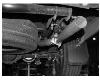
INSTALL PASSENGER SIDE TAILPIPE #C INTO MUFFLER AT LEAST 1 ½" TO 2". USE CLAMP #G TO SECURE PIPE TO MUFFLER. DO NOT TIGHTEN. THE TAILPIPES WILL BOTH LEAN TOWARDS THE DRIVER SIDE. LOOKING FROM THE REAR OF THE VEHICLE - THIS TAILPIPE IS AT APPX. 11 O'CLOCK.
