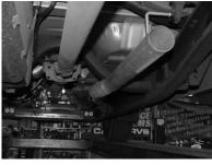
INSTALL MUFFLER #B ONTO HEADPIPE AT LEAST 1 ½" TO 2". USE CLAMP #F TO SECURE MUFFLER TO HEADPIPE. DO NOT TIGHTEN. USE A JACK STAND TO SUPPORT THE MUFFLER. OUTLETS SHOULD BE AT THE TOP. INSTALL HANGER #I ONTO DRIVERSIDE
