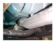
Lay out the exhaust on the floor so it looks like the drawing and compare parts with manual. To remove the stock exhaust Remove it from the stock 2-bolt flange located just behind your catalytic converter. Leave all rubber grommets in place. Use WD-40 to aid in removal of exhaust and hangers. Do not discard your factory hardware. You will reuse your stock bolts.
