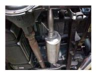
Install the over axle tailpipe #C into the muffler 1-1/2" to 2". Secure to the muffler using clamp # F. Do not tighten.
