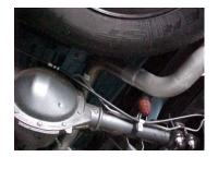
Insert welded hanger into rubber grommet.
