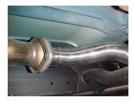
Install head pipe #A on to your existing stock 2-bolt flange using your factory hardware. Use a jack stand to support the converter. Insert welded hanger into rubber grommet. Do not tighten.
