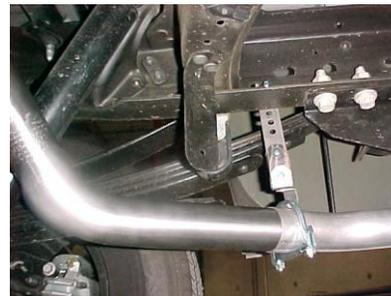
NEXT, INSTALL EXIT PIPES #E ONTO OVERAXLE PIPES. USE CLAMPS # I TO SECURE EXIT PIPE TO OVERAXLES. CUT EXIT PIPES TO DESIRED LENGTH.
