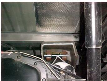
NEXT, LOCATE THE SLOTTED HOLES LOCATED APPROXIMATELY 16" FROM THE REAR OF THE FRAME. MOUNT THE 10" STRAP HANGERS #J INTO THESE SLOTS USING THE HARDWARE KIT # J. MOUNT USING THE 2<sup>ND</sup> HOLE FROM THE TOP.
