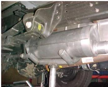
NEXT INSTALL BAND CLAMP #G. SLIDE IT OVER THE MUFFLER. THEN INSTALL HANGERS INTO THE RUBBER GROMMETS LOCATED ABOVE THE MUFFLER OUTLET. USE BOLT KIT # K TO SECURE. DO NOT TIGHTEN.
