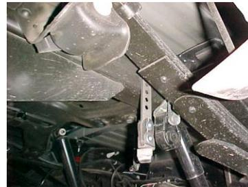
INSTALL PASSENGER SIDE OVERAXLE PIPE #C INTO MUFFLER 1 1/2" TO 2". USE CLAMP # I TO SECURE. DO NOT TIGHTEN. ROTATE UNTIL PIPE TOUCHES HANGER. USE CLAMP #I TO HOLD PIPE TO HANGER. DO NOT TIGHTEN.
