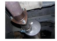
SLIDE MUFFLER ONTO THE FRONT HEADPIPE WITH THE INLET TOWARDS THE CONVERTER (MUFFLER INLET IS LOOKING INTO LOUVERS). USE THE JACK STAND TO SUPPORT THE MUFFLER AND CLAMP USING #G. DO NOT TIGHTEN.
