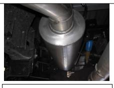
3. Install muffler #B onto headpipe 1.5" to 2" muffler outlets should be on top and level use clamp #G to secure together. Do not tighten. Insert hangers into rubber grommets
