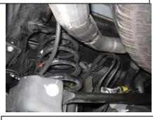
4.Next install Drivers side overaxle tailpipe #C into muffler 1.5" to 2" use clamp #F to secure pipe to muffler do not tighten
