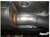
Figure 2: measure 5" inches from behind the passenger side muffler and cut
