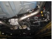
5. Install driver side tailpipe/ dual tip assembly #B. Insert all grommets. Secure tailpipes with clamp #D. Do not tighten
