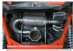
6. Install the Gibson Exhaust reusing the factory springs and gasket. Secure everything in place by loosely fitting the hanger hardware. Install two opposing springs and re tighten the lower hanger points. Now install the remaining two springs.
