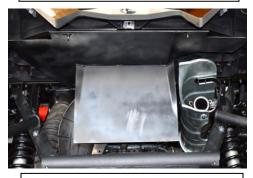
5. Install The Gibson provided under bed heat shield. There are four existing mounting points under the bed. You will loosen the four bolts up install the plate and re install the factory hardware. Check clearance for rattles and tighten down.
