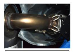
3. Remove the four exhaust springs that connect the muffler to the factory head pipe. Once you have removed the spring's un-bolt the muffler from the two hanger connections located below the muffler. You will re use all hardware.
