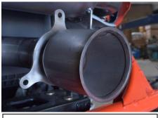
4. Re Install your Factory spark arrestor and tip onto the Gibson Exhaust using the factory hardware. You may need to re adjust the angle once installed on the vehicle with the factory beauty plate.
