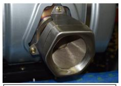
2. Next remove your factory Spark arrestor and tip from your factory exhaust. This will be re used on your Gibson exhaust. Do not damage.
