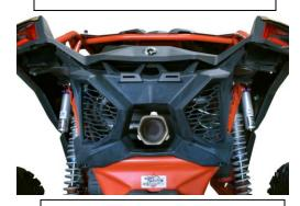
7. Re install the factory exhaust cover. You may need to loosen tip as you install the exhaust to find the right fit. Be sure you have clearance from all components and now drive. After your first ride please double check all clearances and re tighten all components.
