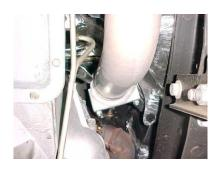
INSTALL DOWN PIPE #K ONTO TURBO USING YOUR FACORY CLAMP. LEAVE LOOSE. DO NOT TIGHTEN.
