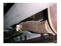
LAY OUT THE EXHAUST ON THE FLOOR SO IT LOOKS LIKE THE DRAWING AND COMPARE PARTS WITH MANUAL. TO REMOVE THE STOCK **EXHAUST REMOVE IT** FROM THE CLAMP LOCATED JUST IN FRONT OF THE MUFFLER. YOU MAY NEED TO HEAT IT UP FOR EASIER REMOVAL. LEAVE ALL RUBBER GROMMETS IN PLACE. USE WD-40 TO AID IN THE REMOVAL OF EXHAUST AND HANGERS.
