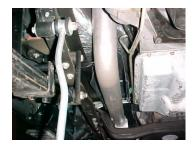
INSTALL DOWN PIPE #L ONTO PIPE #K. USE CLAMP #I TO SECURE PIPES TOGETHER. DO NOT TIGHTEN.
