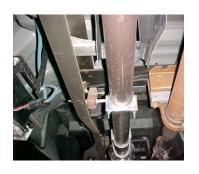
AFTER THIS STEP IS DONE, INSTALL YOUR CAT-BACK SYSTEM THEN YOU WILL ADJUST AND TIGHTEN ALL CLAMPS.
