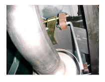
Install band clamp # G into rubber grommets located just above the axle. Do not tighten.
