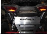
4. Install rear Gibson beauty plate. Use the factory bolts to install. Once they have been installed tighten the Gibson brackets at the rzr frame. Adjust plate for a level finish.
