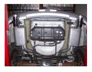
4. Now install the passenger side muffler assembly #C by sliding the metal hangers into the rubber grommets. Then do the same for the driver side muffler assembly #D.
