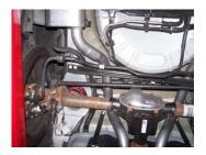
6. Now do the same procedure for the driver side tailpipe #B. Use clamp #E to secure the tailpipe to the muffler assembly and the stock clamp to secure it to the stock h-pipe.
