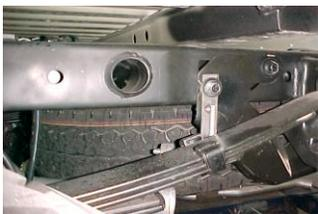
ON DRIVER SIDE: ATTACH REAR TAILPIPE HANGER #I TO FRAME BY REMOVING THE 18MM HITCH BOLT. THEN RE INSTALL BOLT WITH HANGER (IF YOU DO NOT HAVE A FACTORY HITCH USE BOLT KIT #L TO ATTACH HANGER #I TO THE FRAME RAIL. REPEAT ON PASSENGER SIDE.
