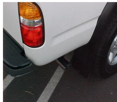
NEXT INSTALL THE STAINLESS STEEL TIP TO YOUR DESIRED LOOK. USE ANY ALUMINUM OR STAINLESS CLEANER TO CLEAN TIPS. NOW GO BACK AND CHECK ALL CLEARANCES AND TIGHTEN ALL CLAMPS.
