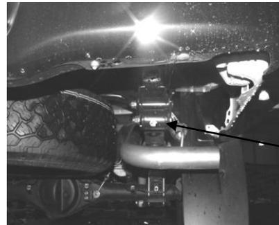
INSERT HANGER INTO RUBBER GROMMET.
