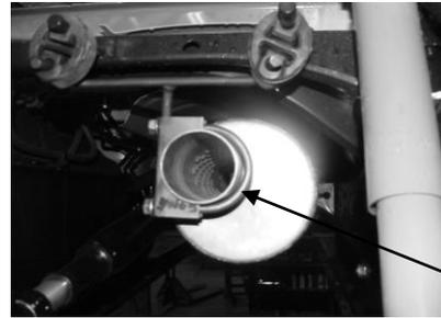
INSTALL REAR MUFFLER HANGER #F AT THE REAR OF THE MUFFLER AND ATTACH TO RUBBER GROMMETS. THE VERTICAL ROD WILL BE AIMING UP ON THE DRIVER SIDE OF THE VEHICLE.
