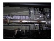
3. Install headpipe #A onto your existing stock 2-bolt flange. Use bolt kit #G to secure. Do not tighten. Insert welded hangers into rubber grommets.
