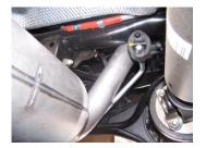
5. Install the over axle tailpipe #C into the muffler 1.5-2". Secure to the muffler using clamp #F. Do not tighten. Insert welded hanger into rubber grommet.
