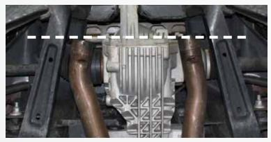
You will need to cut the mufflers from the vehicle using a hack saw or sawsall. Line up your cut with the end of the Rear Differential.
