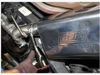
Starting at the inlet pipe clamp adjust the axle back system to your personal preference and tighten the clamps
