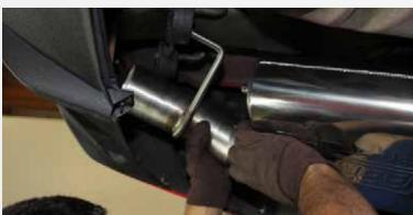
Slide the exit pipe onto the muffler and through the rear hanger grommets, then snug the clamp enough to still allow adjust-ability.
