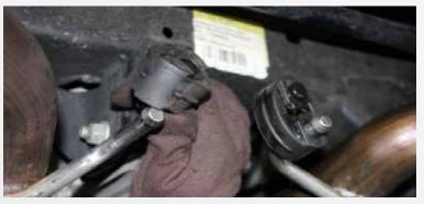
Remove the inner rubber grommets holding the muffler hangers.
