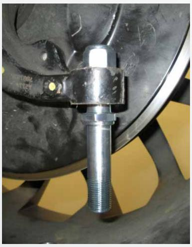
Insert the tapered end of the tie rod stud into the spindle and tighten it using the supplied hardware. After insuring that the wheel is still centered and after tightening the tie rod stud you will need to adjust the Gripp Adjuster Sleeve so the outer tie rod end lines up with the rod stud. Once proper alignment is achieved tighten the Jam nut.
