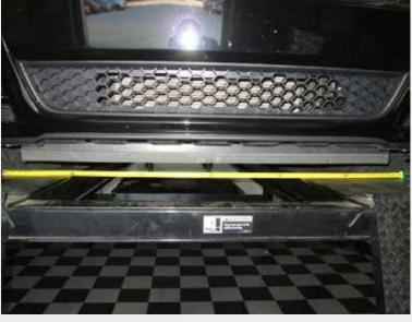
In order to get proper "Rough" measurements this installation MUST be done on a drive on lift or drive on ramps, that way the alignment and tie rod angles are close enough to how it was before the installation so that the vehicle can be driven to the performance alignment shop.
