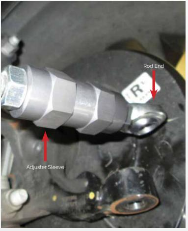
Thread the Gripp Adjuster Sleeve onto the inner tie rod, and then thread the supplied Rod End into the Adjuster Sleeve all the and tighten the jam nut.
