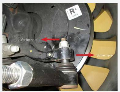
Loosen the top nut of the tie rod end. Using a steel hammer, gently strike the side of the spindle until the old ball joint stud falls out. If the stud still doesn't break loose then thread the nut back on to the stud enough to cover the threads and strike the top of the stud.
