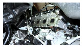
18 Any carbon build up should be removed gently with a small putty knife – DO NOT scratch the head surface!
