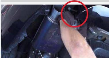
Slide the muffler over the inlet pipe, then slide the grommet closest to the rear bumper onto the muffler hanger.
