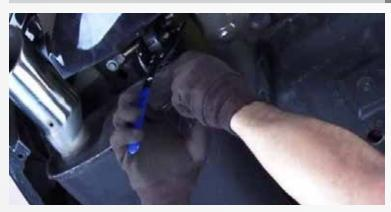
Using a pry bar or grommet removal tool, remove the rubber grommet located by the muffler tip from the muffler hanger.
