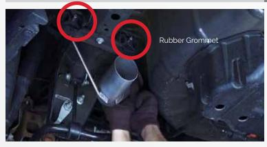
Starting on the driver side, slide the inlet pipe through the 2 hanger grommets and into the mid pipe and snug the clamp to hold the tubing in place.
