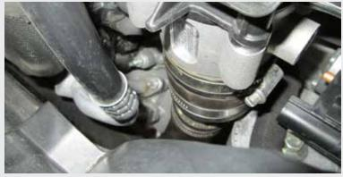
Now reverse all processes installing BBK throttle body, alternator wire, intake tube, chassis cover, etc.
