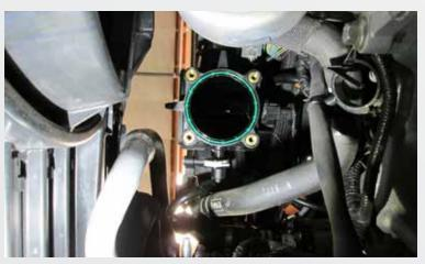
Disconnect signal plug from throttle body then using 8mm socket and extensions remove factory throttle body.
