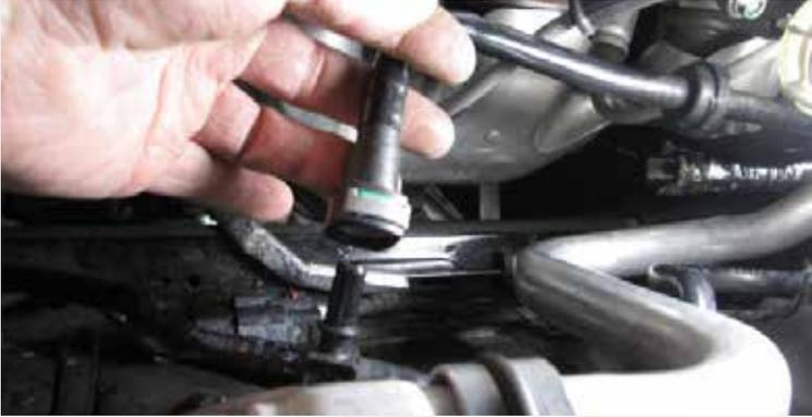
Disconnect the (2) rubber mounting straps that hold the sound tube to the strut brace and A/C line located on the driver side of the engine. Below the A/C line there is another vacuum line with a quick disconnect fitting disconnect that vacuum line and push it towards the fire wall then toward the driver side inner wheel well so that it is tucked out of the way.
