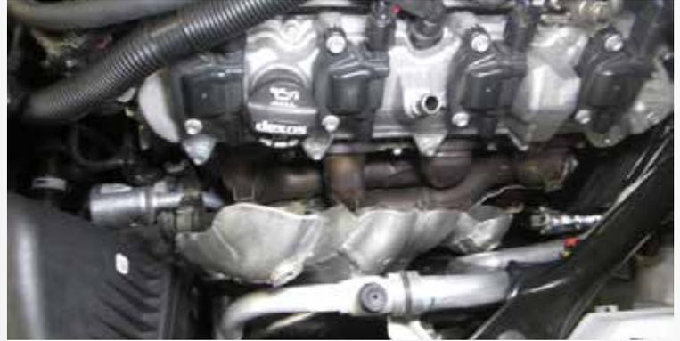
Remove the (3) bolts that hold the heat shields to the exhaust manifold on the driver and passenger side of the engine and remove the heat shields from the vehicle.
