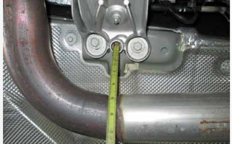
Remove the (2) bolts that hold the connect rod for the steering shaft. Once the (2) bolts are removed push the connecting rod towards the fire wall until the connecting rod releases from the rack and opinion end then you may slid the connecting rod towards the front of the vehicle to release it from the steering shaft and remove it from the vehicle.
