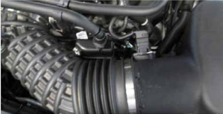
Disconnect the mass air flow sensor from the air inlet tube. Disconnect the vacuum tube located next to the mass air flow sensor. Using pliers disconnect the sound tube from the barb fitting located on the top of the air inlet tube. Loosen the clamp that holds the air inlet tube to the throttle body. Unclip the sound tube from the side of the air box. Disconnect the inlet tube from the throttle body and lift up on the air box to release it from its mounting points and remove it from the vehicle.
