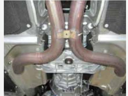
From underneath the vehicle take a measuring tape to use as a guide line to mark where the exhaust will be cut. Stick the end of the measuring tape into the hole in between the (2) transmission cross member bolts and hold it straight up and down and mark the exhaust pipe on the side of the tape measure that is closest to the front of the vehicle do this on the driver and passenger side of the exhaust. Using a saw's all cut the exhaust pipes where you had made the marks.
