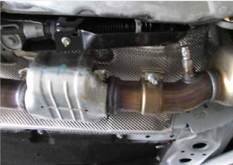
Remove the (4) bolts that hold the catted down pipe to the collector on the exhaust manifold do this for both driver and passenger sides. Support the exhaust system so that it does not fall down. Remove the (4) bolts from the exhaust cross member bracket and remove it from the vehicle. Release the exhaust system to let it drop down and rest on the chassis cross brace.
