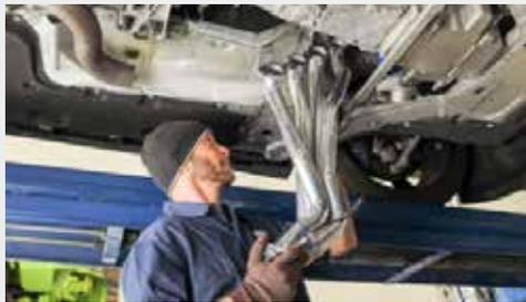
On the passenger-side of the engine. Remove the bolt that holds the dipstick to the cylinder head. Remove all exhaust manifold bolts.
