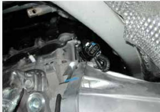
Utilizing approved jack and jack stands or preferably a vehicle hoist lift the vehicle as high as possible and secure the vehicle properly. Disconnect the (4) oxygen sensor's from the wire harness.
