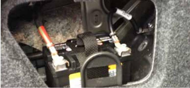
Disconnect the negative battery terminal from the battery located in the truck on the passenger side. Place a rag over the trunk latch so the trunk lid will not latch with the battery disconnected.
