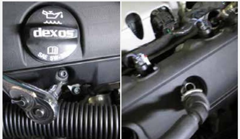
Remove the (2) Torx bit screws on the driver and passenger side coil covers. On the driver side remove the oil cap. Disconnect the vacuum tube that goes into the valve cover on the driver side and passenger side. Once the vacuum tubes are off lift up on the coil covers and remove them from the vehicle. Replace oil cap so no debris will enter the engine.
