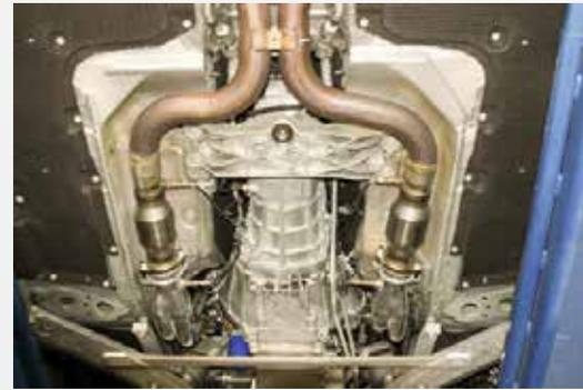
Install all (4) oxygen sensors and connect the wiring harnesses. Reconnect the negative battery terminal and enjoy the sound and power of the BBK full length headers "REMINDER" check coolant levels after
