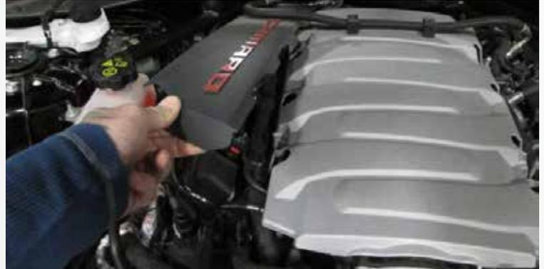
Remove the engine decorative covers from the engine by simply pulling them upwards released them from their mounting points.
