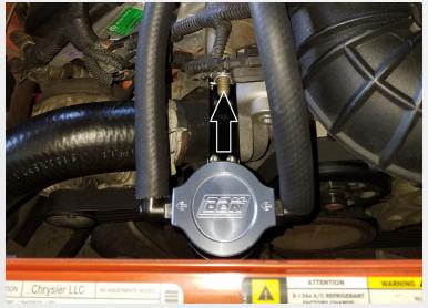
Bolt the BBK oil separator bracket to the engine block using the supplied bracket and hardware, install the BBK oil separator onto the bracket as shown in the picture.
