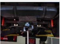
Support the fuel tank and remove the tank retaining straps.
