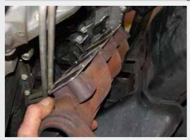
Unbolt both exhaust manifolds and remove from the vehicle. Also remove the stock gaskets.
