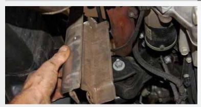
Remove the four nuts that hold the heat shields to the exhaust manifolds and remove them.
