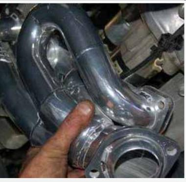
On the driver side, the steering shaft needs to be unbolted and moved to the side and the engine needs to be lifted. Install the supplied gasket and BBK Header into place and tighten in an X-pattern.
