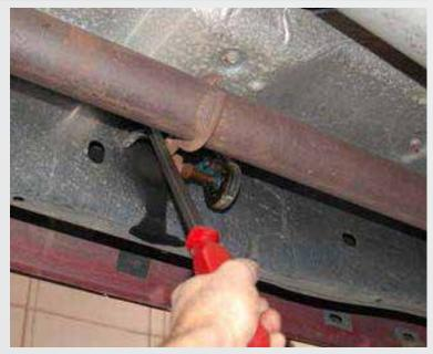
Unbolt the downpipes/cats from the exhaust manifolds. Using a pry bar, slide the whole exhaust system back on the metal rod hangers. Move it back far enough that the exhaust manifolds can be removed. It just takes a few inches and its out of the way.
