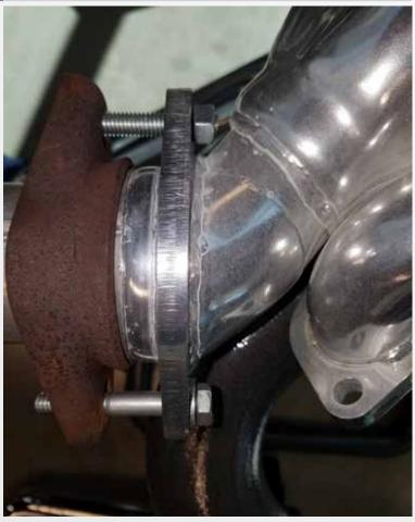
Now work the exhaust forward: torque the headers and installed supplied hardware. Notice in the picture on driver-side we supplied 1pc X 2 inch long bolt and 3pcs X 2  $\frac{1}{2}$  Inch long bolts. Use the shorter 2 inch on the in-side of the elbow area. Now tighten exhaust down evenly and re-connect O2 sensor plugs.
