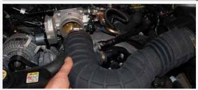
Disconnect the breather tube from the air intake tube. Loosen the clamps at the throttle body and at the air box then remove the air intake tube.
