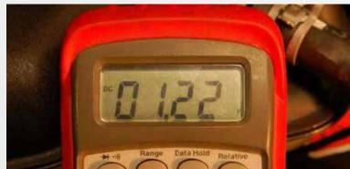
MUSTANG Probe the top wire of the TPS Sensor.
