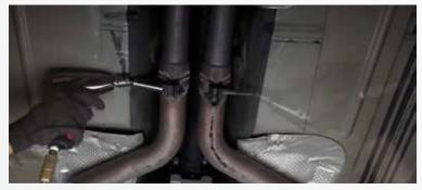
Remove the nuts that attach the H-Pipe to the factory manifolds.
