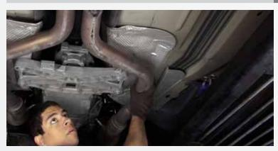
Push the H-Pipe forward to meet up with the BBK Headers and tighten the collector flanges using the supplied washers and nuts. Then tighten the H-Pipe clamps.
