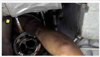
Install the BBK headers by sliding the slots onto the started bolts (over the gaskets) then inserting and tightening all of the supplied header bolts.
