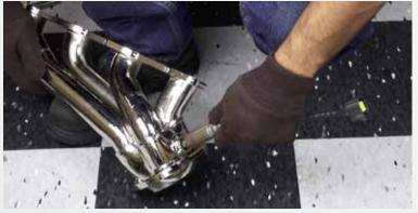
Transfer the oxygen sensors from the factory exhaust manifolds to the BBK Parts.
