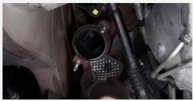
Remove the heat shields from the motor mounts and the factory exhaust manifolds.
