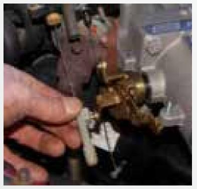
Re-install the throttle cables and return spring.
