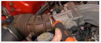
Remove the Air Temperature Sensor from the inlet tube. Loosen the clamps on the inlet tube at the throttle body and at the air box. Disconnect the breather hose and remove the inlet tube.
