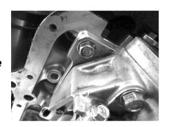
Clearance between the notch of the pan and the subframe may cause fitment issues. This issue has two possible solutions. The first solution is to grind the subframe to allow for proper clearance between the pan and the frame. We understand that this may not be a favorable option for all. Motor mount spacers can also be used to raise the motor and allow for proper clearance.
