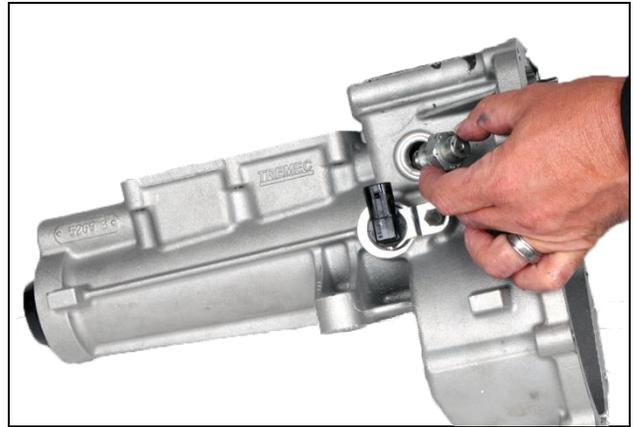
7.6: Install shift rail detent. Torque to 25-35 lb-ft
