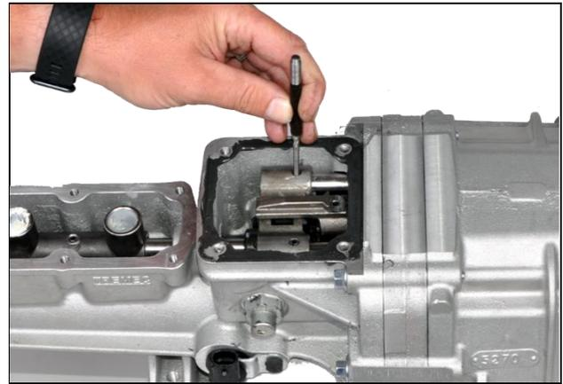
**3.7:** Use a pin punch to remove three roll pins holding the shift lugs
