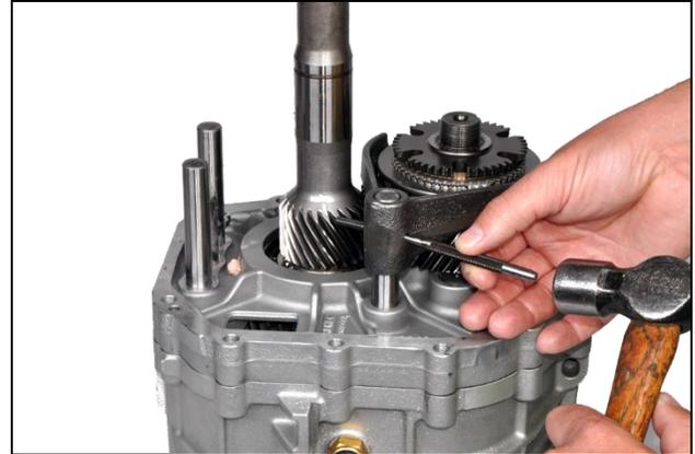
**3.23:** Remove 5<sup>th</sup> gear fork roll pin
