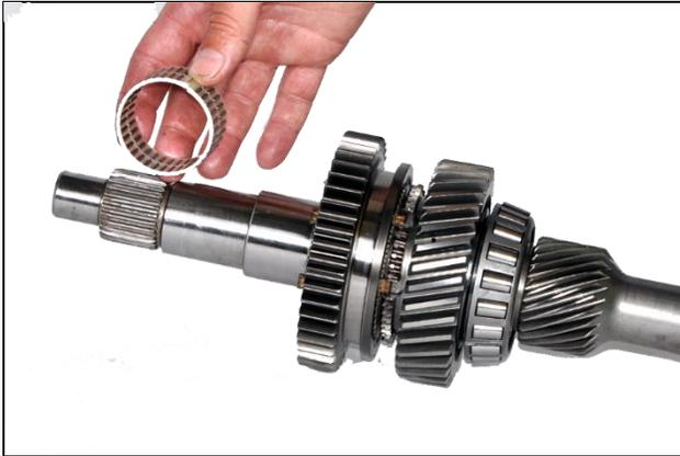
**6.11:** Install 2<sup>nd</sup> gear bearing onto main shaft
