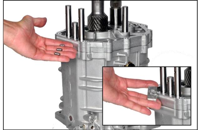
**8.14:** Install shift rail interlock pins (three pieces)
