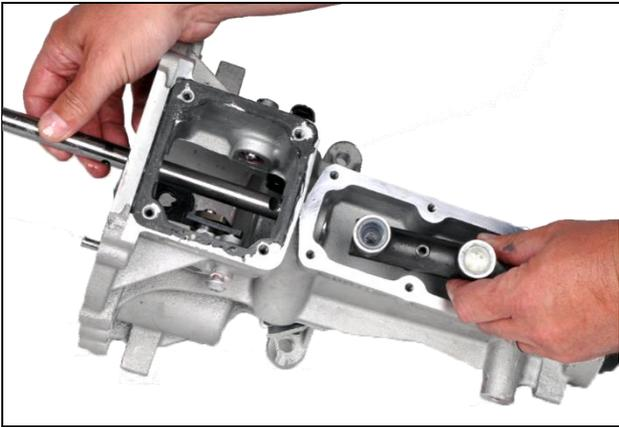
7.4: Install roll pin for shift lever socket
