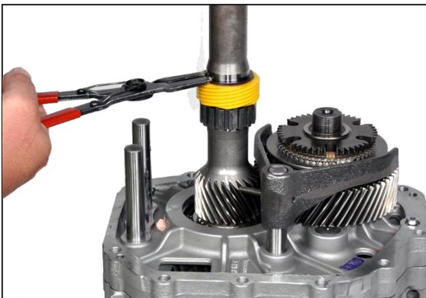
**3.18:** Remove speedometer gear snap ring
