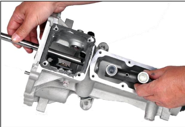
4.4: Remove roll pin from shift lever socket
