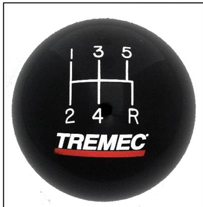
The TREMEC 5-speed TKX manual transmission has five forward gears plus reverse. The gear patterns are clearly marked on the shifter or dashboard.
