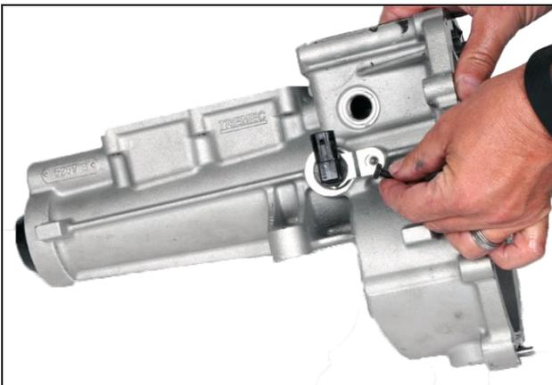
4.7: Remove bolt from Vehicle Speed Sensor (VSS)
