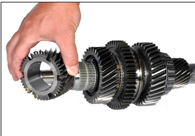
**6.15:** Install 3<sup>rd</sup> gear onto main shaft
