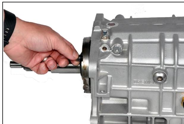
**8.30:** Install four bolts. Torque to 12-16 lb-ft.
