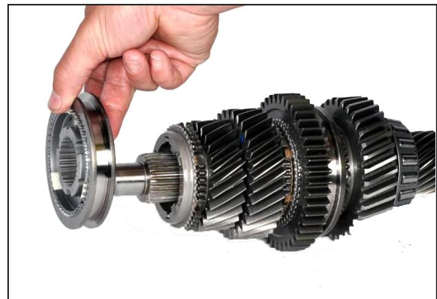
**6.16:** Install 3<sup>rd</sup> gear blocking ring
