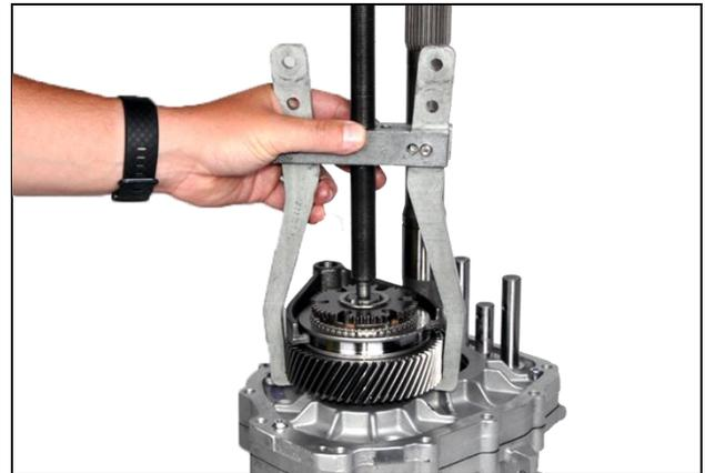
**3.26:** Using a two-jaw puller, remove 5<sup>th</sup> gear and synchronizer assembly
