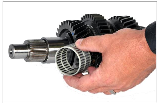
**6.14:** Install 3<sup>rd</sup> gear roller bearing and bearing thrust sleeve onto main shaft
