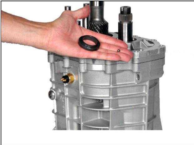
**8.16:** Install 5<sup>th</sup> gear bearing and thrust washer to cluster shaft
