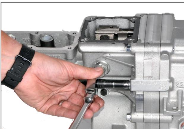
**3.8:** Remove 11 extension housing-to-transmission case retaining bolts
