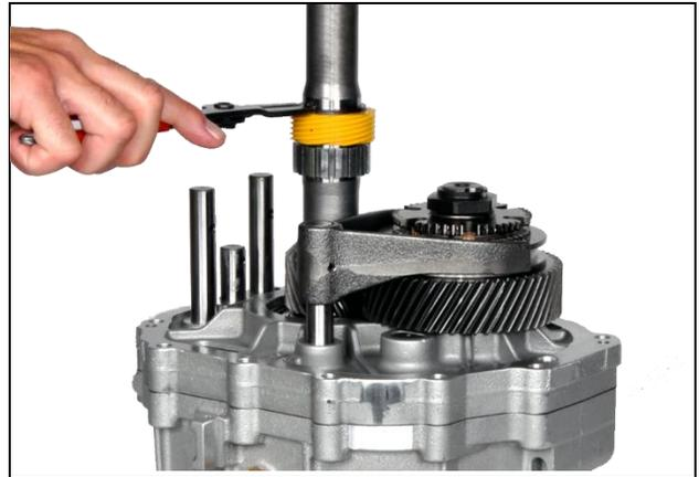
**8.24:** Install speedometer gear snap ring
