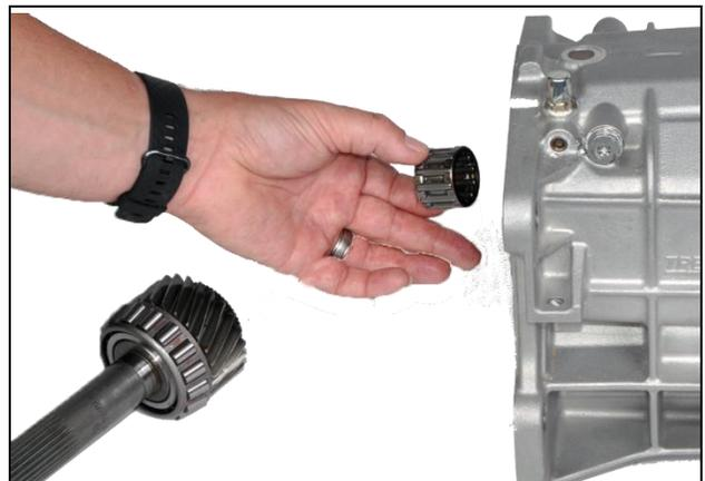
**8.28:** Install input shaft and pocket bearing
