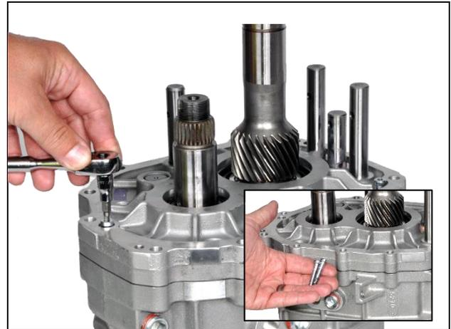
**8.17:** Install bolt into intermediate plate (two pieces)
