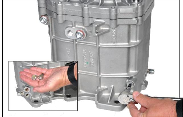
**3.38:** Remove two shift rail detent plugs
