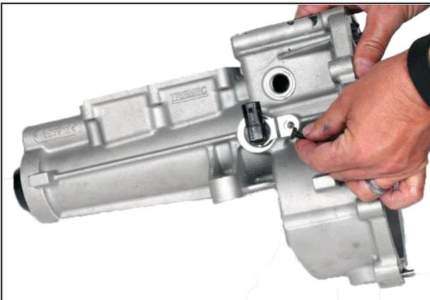
7.7: Install bolt for Vehicle Speed Sensor (VSS)
