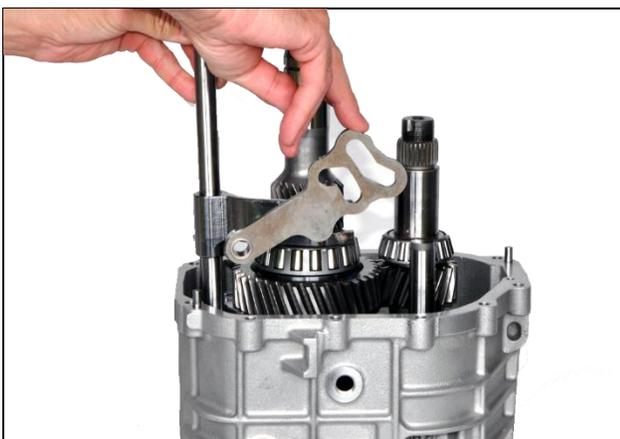
**8.5:** Install 5<sup>th</sup> and reverse gear selection arm into case
