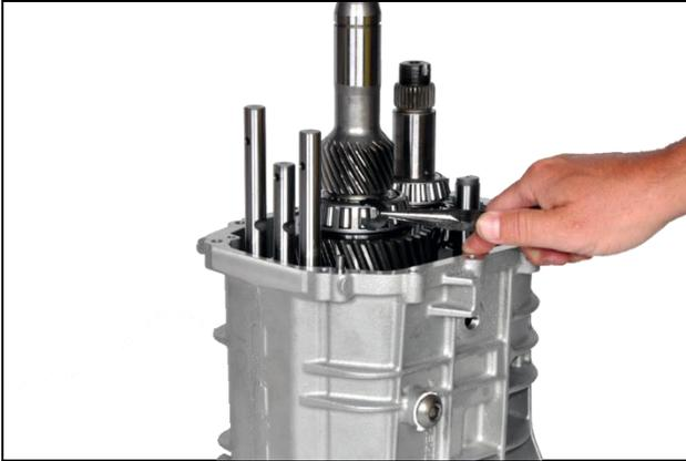
**8.7:** Install pivot pin snap ring
