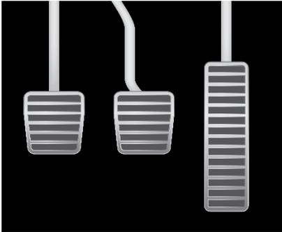
A manual transmission requires the driver to shift the gears themselves. It will have three pedals: clutch, brake and accelerator to operate the vehicle.
