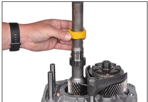
**3.19:** Remove mechanical speedometer gear
