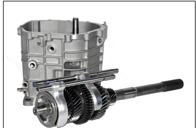
**8.2:** Install 1-2 and 3-4 shift forks and rails onto main shaft
