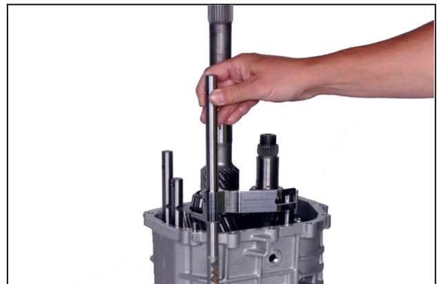
**8.4:** Install 5<sup>th</sup> and reverse gear fork and rail into main case
