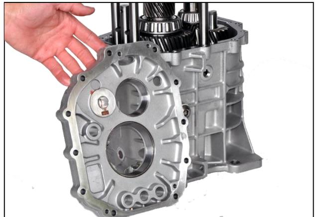
**8.12:** Install rear housing gasket and intermediate plate. (Note: Be careful to line up idler gear thrust washer.)
