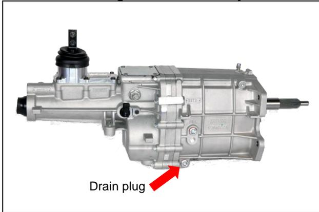
**3.1:** Start tear down by setting transmission on a sturdy bench
