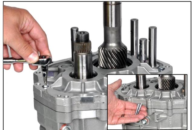
**3.29:** Remove two mid-plate retaining screws
