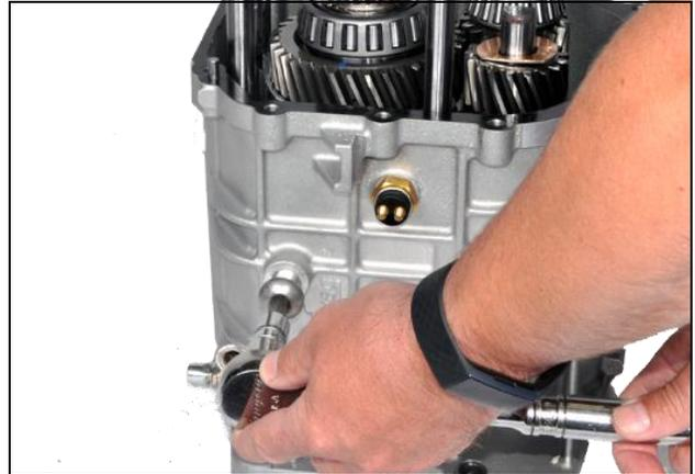
**3.33:** Remove selector link pivot bolt
