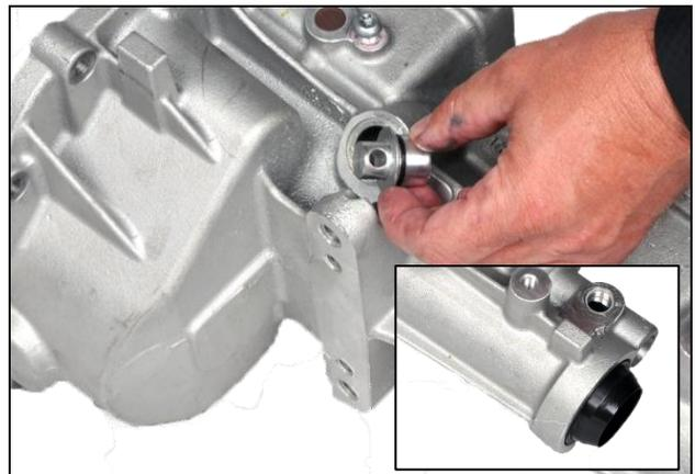
4.9: Remove bolt from mechanical speed plug
