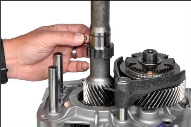
**3.21:** Remove electronic speedometer gear
