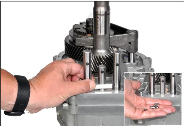
**3.24:** Remove hold down block from shift rails
