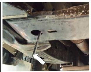
Note: Feed nut plates through slot openings located on underside of rear cross member.
