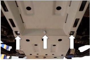
17. Loosely fasten transmission panel to diff panel using 3x M8x25mm bolts, 3x M8 spring washers, 3x M8 flat washers and 3x M8 flange nuts.
