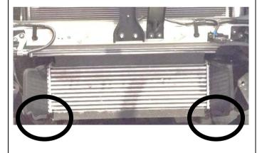
3. Trim lower section of air deflectors located on each end of intercooler by an even 10mm.
