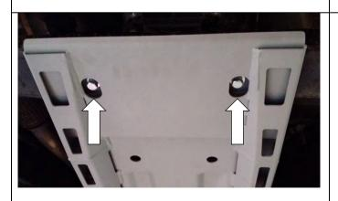
16. Loosely fasten transmission panel to chassis cross member using 2x M10x35mm bolts, 2x M10 spring washers, 2x M10 flat washers and 2x M10 nut plate.
