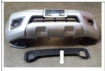
1. Remove dressing piece from lower section of bumper (leave bumper attached to vehicle).
