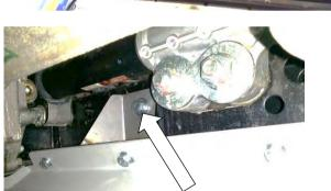
13. Fasten M10 nut plate at rear of front panel to chassis using an M10x35mm bolt, M10 spring washer and M10 flat washer and tighten all M8 and M10 fasteners.
