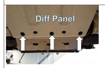
15. Loosely fasten diff panel to front panel using 3x M8x25mm bolts, 3x M8 spring washers and 3x M8 flat washers.
