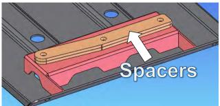
14. Loosely fasten diff panel to underside of chassis using 3x M10x70mm bolts, 3x M10 spring washers, 3x M10 flat washers and 3x M10 flange nuts.
