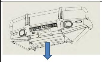
8. Remove ARB stone guard and retain all M6 and M8 fasteners removed.
