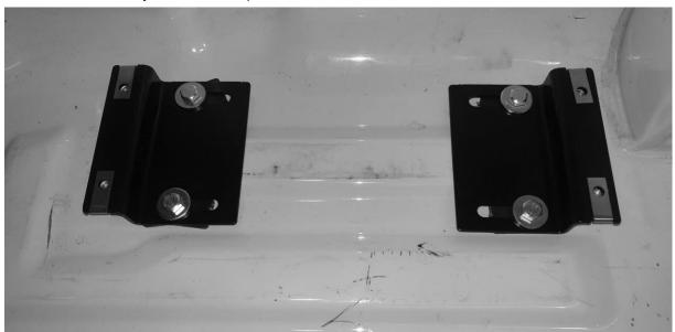
After the accessories have been fitted re-attach the assembled compressor mount to the feet using 4 X M6 X 20 HXHD bolts and 4 X M6 X 20 X 1.6mm flat washers and tighten the M6 fasteners to 9Nm [7lbf.ft]
