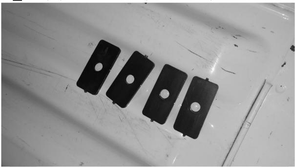
Place the packers in valleys and position universal compressor mount in the required location.
