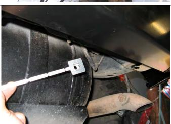
11. Place cage nut plates on inside of cross member for outer drilled holes and secure using M10 x 35mm bolts, spring washers and flat washers. Once this is complete tighten bottom chassis bolts first followed by all other fasteners.
