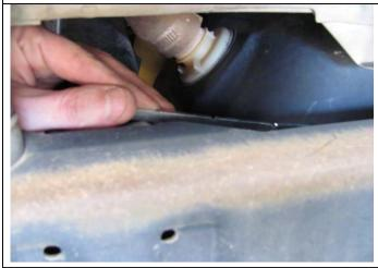
6. Feed LH side cage nut plate over top of chassis and behind fuel tank. Adjust the end with the M10 cage nut so it will sit flat with the drilled centre hole on the LH side.
