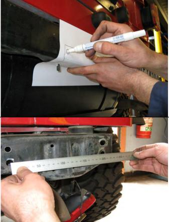
3. Place the drilling template over the existing studs on bottom of chassis and wrap around cross member as shown. Mark the two holes on the rear face using a white marker and then centre punch. Drill a pilot using a 6mm drill bit then enlarge to 14mm (9/16). De-burr and paint holes when done.
