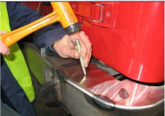
13. If fitting fog light punch out 2 mounting holes in bar as shown.
