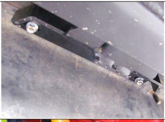
12. Re-fit two centre tank guard nuts. Do not over tighten. If centre studs are in bad condition or broken do not be alarmed as these are not critical for bar fitment.
