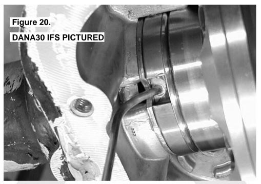
NOTE: The seal housing tube should lay as low in the seal housing groove as possible.
