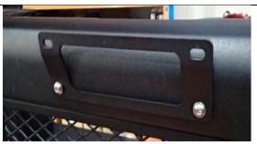
27. Fit number plate and bracket to upper pan using 4xM6x16 dome head bolts, flat washers and flange nuts.
