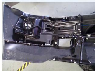
7. Remove the reinforcing from behind the OE bumper. Remove the original wiring loom and park sensors. Remove park sensors by spreading tabs apart and sliding sensors out the back face of the bar.
