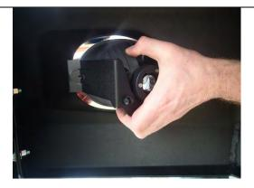
15. Remove globe from fog light by twisting anti clockwise.
