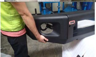
9. Fit the wings to the centre section using the 10x M12 bolts, flat washer, spring washers and flange nuts from the wing fitting kit. Align the wings to the front and top face of the bar as shown.
