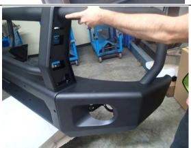
13. If fitting outer frames, use the M12 bolt, flat washer and spring washer provided in the outer frame kit to loosely secure the end of the outer frame to the wing.
