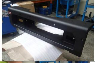
8. Secure the lower centre bar on a sturdy trolley or bench.
