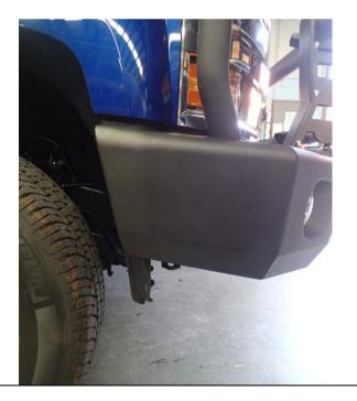
21. Using a suitable lifting device, bring the bar to the vehicle chassis.
