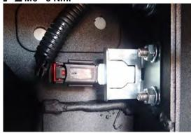
Right hand side outer sensor and bracket
