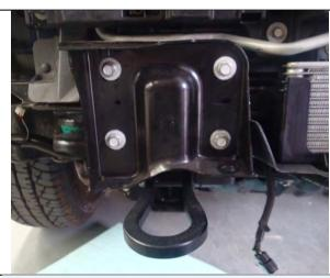
6. Once the bumper is off, remove the original bumper brackets from the chassis, and retain the bolts.
