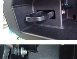
Fit tow hooks and reinforcing brackets into the bar
