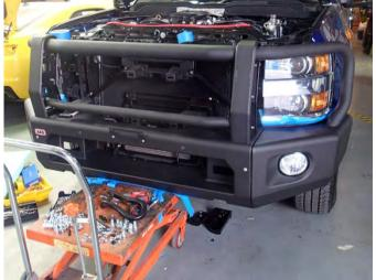
Tape is used under the headlights and under the bar to profect these areas from scratches during fitment.
