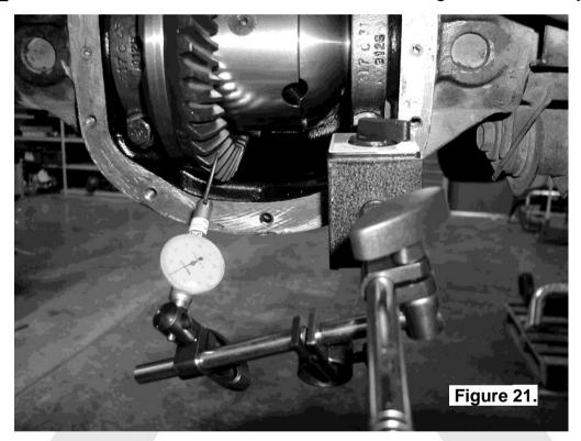
Refer to your vehicle service manual for the specified maximum and minimum amounts of backlash. If the backlash is not within the specifications then the differential will have to be removed and reshimmed.
