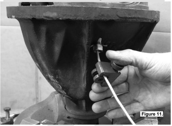
NOTE: Use an automotive brake line tubing cutter to cut the seal housing tube, never a hacksaw as this will leave metal filings in the air system.
