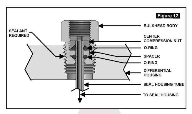
Make sure the seal housing tube is all of the way into the center compression nut while you are tightening it.
